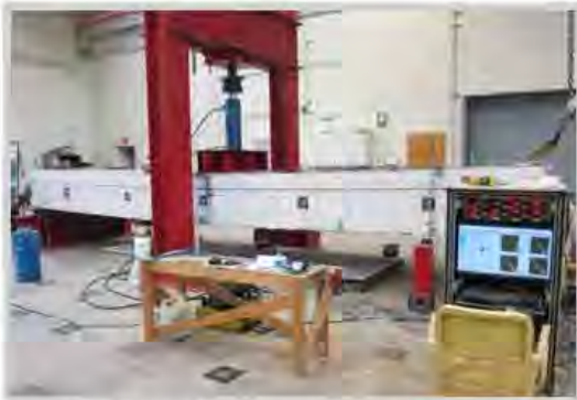
(a) Testing of a full-size concrete box girder
